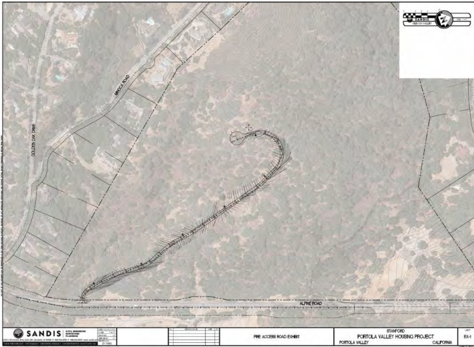
Figure 23 Landing/Staging Area and Access Road for Material Storage and Removal
