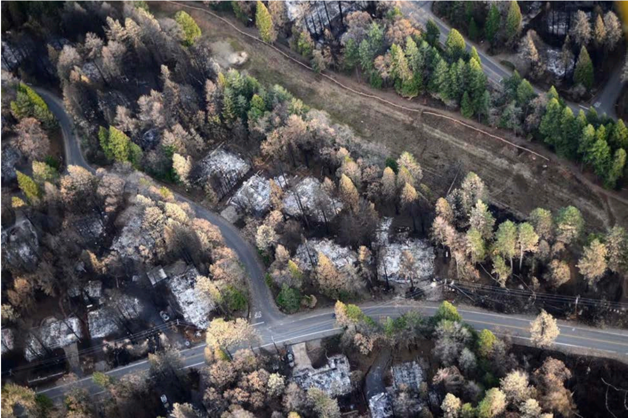
Fig. 4. Canopies don't ignite structures. Rather, structures ignite canopies. While anecdotal, this image from Knapp et al. highlights the effects of intense radiant heat from burning buildings and suggests that, like homes, survival of trees increases the further they are from structures. Reference in endnotes.
