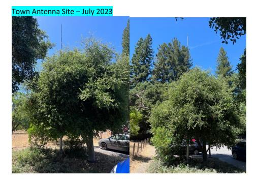
This location is at the southwest corner of the parking lot by Town Hall. This tree was not present when the antenna was originally located. The bulk of the tree covers the top of the mast and the base of the antenna. It will severely impair the performance of any antenna at this location.
