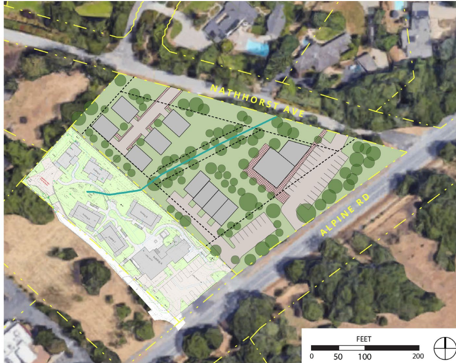
Figure 4: Conceptual Site Plan for 4370 Alpine Road as described in the Housing Element. The rear portion of the site shows 5 detached two-story units with ground-floor individually secured parking. The front portion of the site supports 4 attached two-story units and a commercial building.
