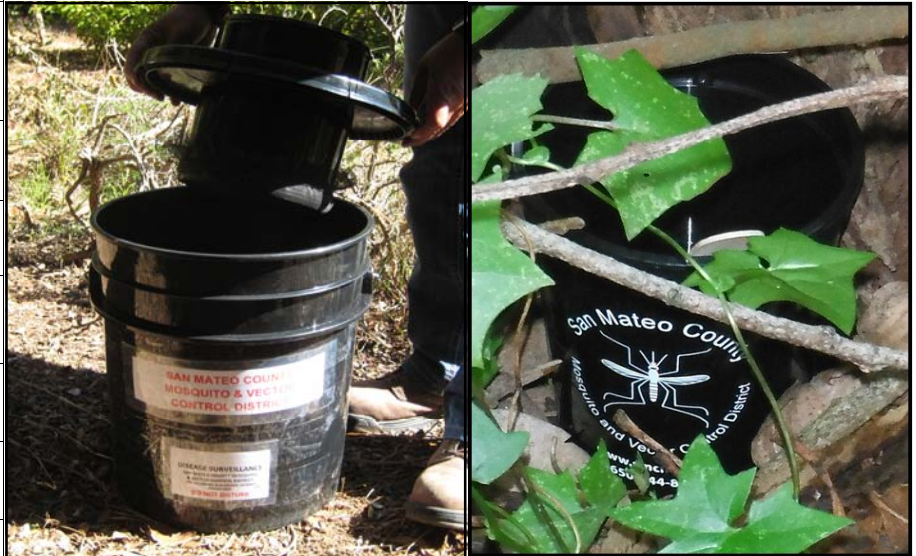
Traps for female Aedes aegypti deployed in Menlo Park and cemeteries throughout the county for the District's Aedes Surveillance Program. The traps are monitored until late fall. From left to right: Autocidal Gravid Ovitrap (AGO) and ovitrap (pint cup).
