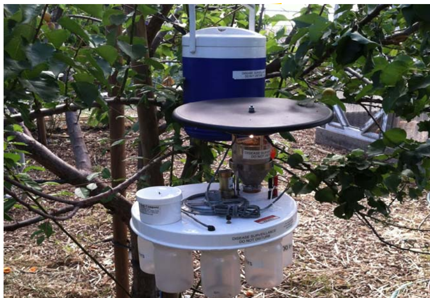
A rotating collector trap for adult mosquitoes undergoes a trial run at the East Palo Alto chicken coop. The trap design reveals the time of day the mosquitoes were caught.
